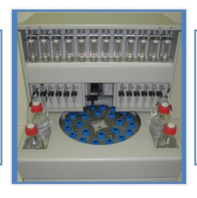
Each reaction vessel has a dedicated pre-activation vessel for more efficient coupling.
