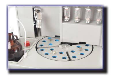
All reagents and solvents are delivered from the top of the reaction vessels.
